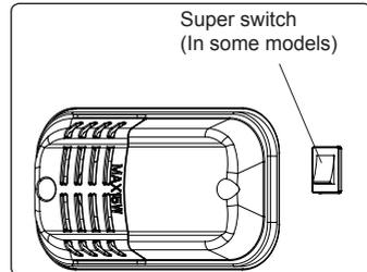
This switch shall be used as superfreeze switch. For maximum freezing capacity, please turn on this switch before 24 hours placing fresh food. After placing fresh food in the freezer, 24 hours ON position is generally sufficient. In order to save energy, please turn off this switch after 24 hours from placing fresh food.
