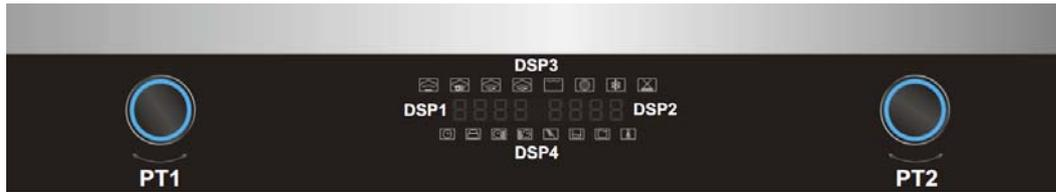
PT1. This button is used to setup time, choose cooking time length, high and low temperature.
