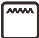
**GRILL:** This method of cooking utilises the inner part only of the top element, which directs heat downwards onto the food. This function is suitable for grilling small portions of bacon, toast and meat etc.
