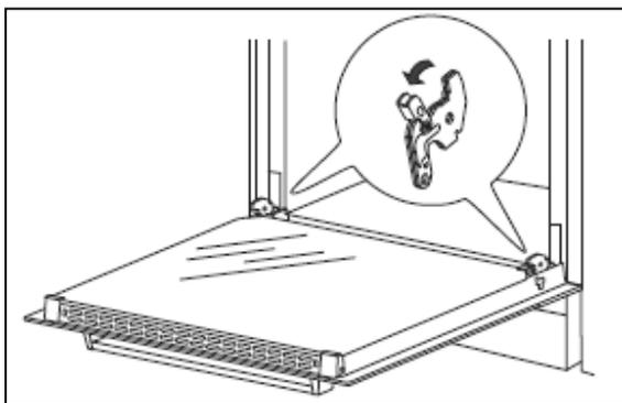
To facilitate the cleaning of the inside of the oven and the outer frame of the oven, the door can be removed as follows:
