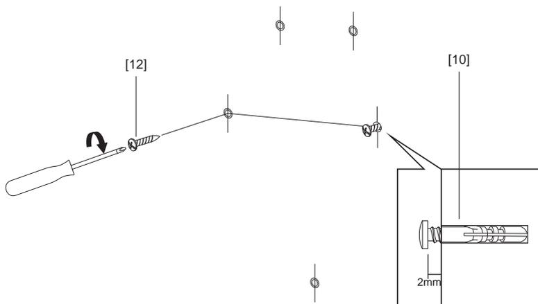
Drill the wall, insert the plugs for all the 6 marked holes and fix the screws for the top two holes of the hood.
