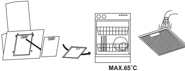
Aluminium filters: to avoid fires, clean thoroughly once a month or whenever the display pilot light indicates as such. To do so, remove the filters and wash with hot water and detergent. If using a dishwasher, position the filters vertically to improve the cleaning process.
