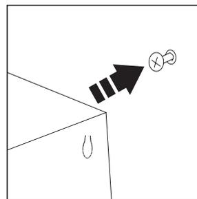
Position the hood over the top two screw then fix the bottom screws from inside the hood.
