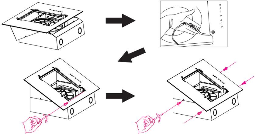
Connect the electric cable and fix the metal box and motor to the glass and metal work.
