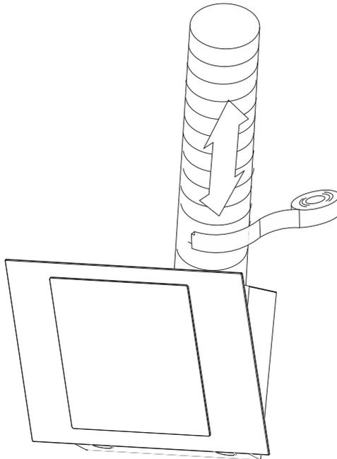
Fix the Ducting Tube 125 or 150 using tape or clamp.
