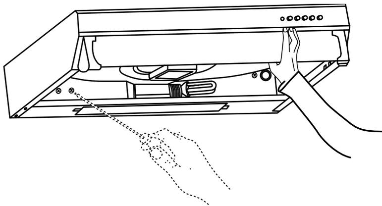
Whilst holding the hood, and tighten inside screws
