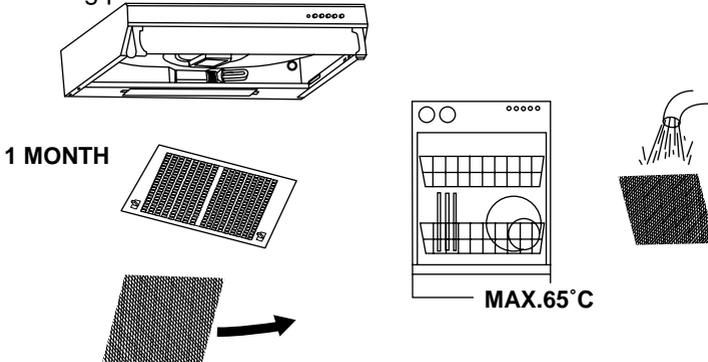
Aluminium filters: to avoid fires, clean thoroughly once a month or whenever the display pilot light (if fitted) indicates as such. To do so, remove the filters, soak in hot water and mild detergent for an hour. If using a dishwasher, position the filters vertically to improve the cleaning process.
