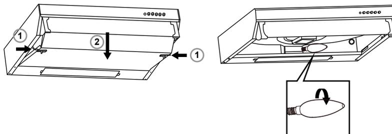
Push the clips (1) inwards and release the metal filter & cover (2).
