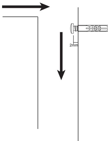
Position hood over 2 wall screws, and use keyhole slots on adjustment bracket to support the weight.
