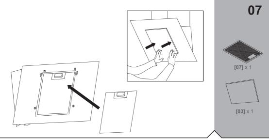
Replace the aluminium filter and fix front glass panel.
