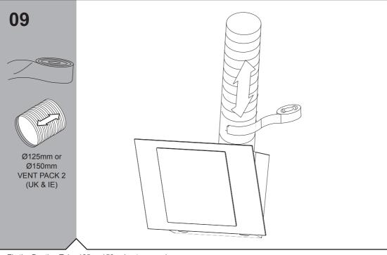
Fix the Ducting Tube 125 or 150 using tape or clamp.
