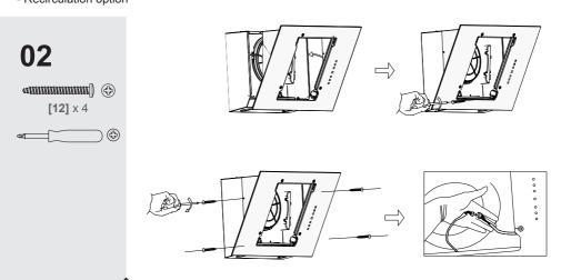
Fit the metal box and motor to the glass and metal work.
