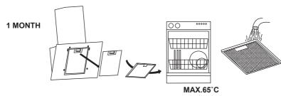
Aluminium filters: to avoid fires, clean thoroughly once a month or whenever the display pilot light indicates as such. To do so, remove the filters and wash with hot water and detergent. If using a dishwasher, position the filters vertically to improve the cleaning process.
