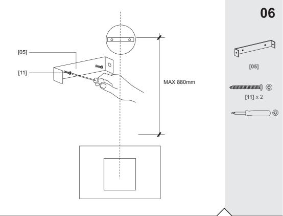
Fix the top bracket to the wall.
