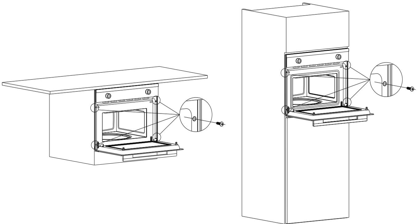
Note: Do not take the door handle as force bearing point during the installation and removal.
