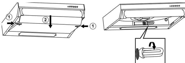
Push the clips (1) inwards and release the metal filter & cover (2).
