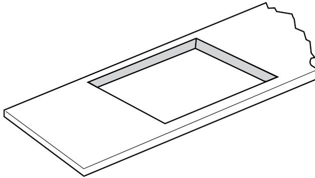
Cut out worktop to the template dimensions with suitable equipment.
