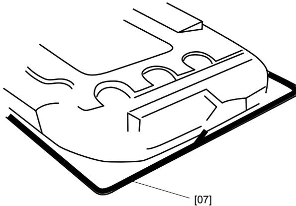
Stretch out the supplied seal along the underside edge of the hob, ensuring the ends overlap.
