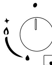
Automatic electric "ON" switch for burners with safety device (thermocouples):
