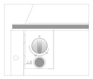
The controls consist of a temperature dial and an On/Off switch. These are only visible when the drawer is open.
