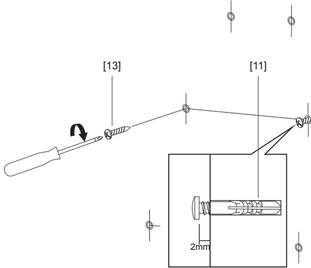
Drill the holes, insert the wall plugs in all 6 holes. Insert the screws in the middle 2 holes in fig.03. Maximum gap between top 2 holes and middle 2 holes can be no more than 935mm, dependant on ceiling height
