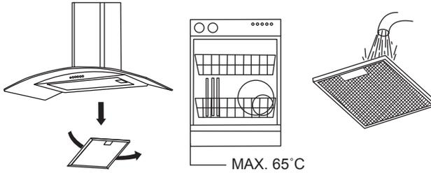
**Aluminium filters:** to avoid fires, clean thoroughly once a month. To do so, remove the filters and wash with hot water and detergent. If using a dishwasher, position the filters vertically to improve the cleaning process.
