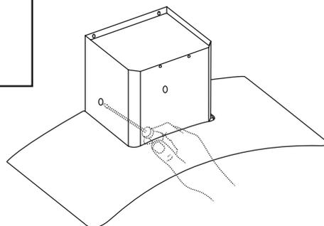
Position the hood over the top two screw then fix the bottom screws from inside the hood.
