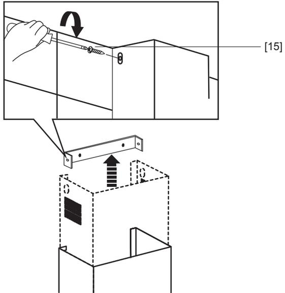
Fit the chimney sections to the bracket. Connect top of the ducting tube to vent kit as per manufacturers instructions.
