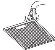
**Aluminium filters:** to avoid fires, clean thoroughly once a month. To do so, remove the filters and wash with hot water and detergent. If using a dishwasher, position the filters vertically to improve the cleaning process.
