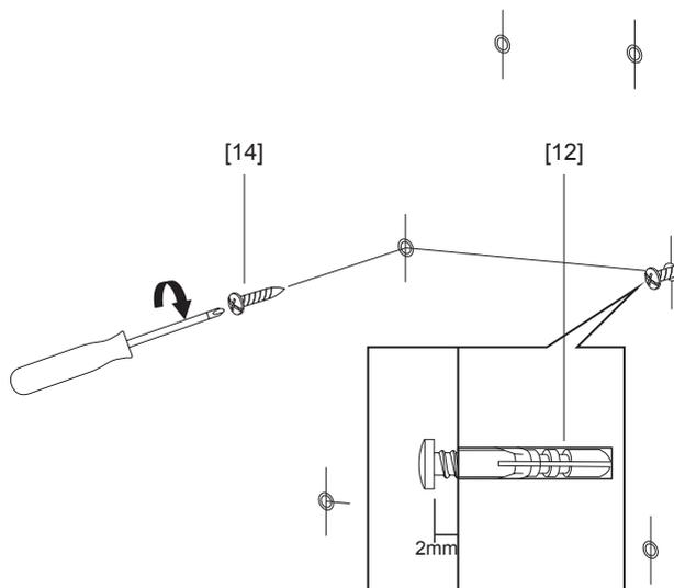
Drill the holes, insert the wall plugs in all 6 holes. Insert the screws in the middle 2 holes in fig.03. Maximum gap between top 2 holes and middle 2 holes can be no more than 855mm, dependant on ceiling height
